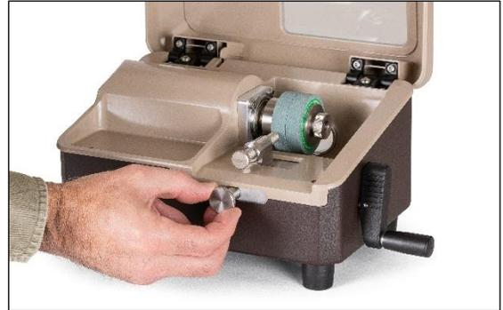
6. Close the hinged safety cover. Turn wheel refacer on by depressing On/Off switch located on rear of instrument. Turn vacuum unit on.
