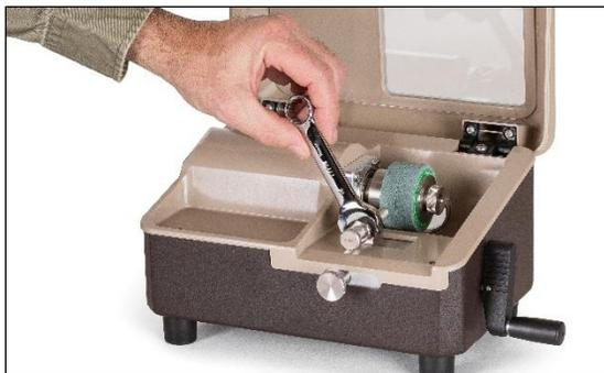
5. To set the diamond tool for a light cut, turn the cut depth adjustment knob clockwise approximately  $\frac{1}{8}$  turn after the diamond tool contacts the wheel. If the wheels are of different diameters, use the larger of the two diameters. If necessary, traverse the diamond tool to the left so it does not contact the wheels.
