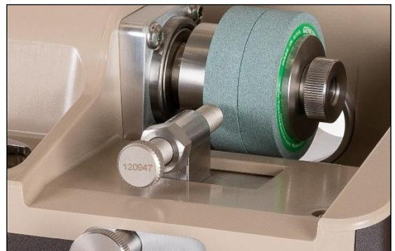
9. After completing the refacing operation, ensure the diamond tool is returned to the start position (left). Remove the wheels from the wheel arbor and reconnect the vacuum hose to Taber Abraser.
