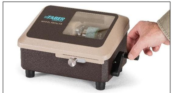
8. Turn the cut depth knob clockwise approximately  $\frac{1}{8}$  turn, then continue refacing until the wheel surfaces have been completely renewed. Repeat if necessary.
