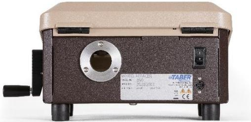
2. Use the hand crank handle to position the diamond tool to the left.
