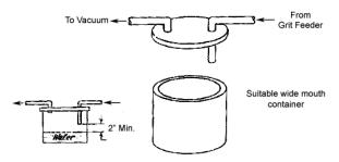
A tight seal is not required between the container and the lid. Also, the inlet pipe to the water trap should be far enough away from the water surface that undue turbulence is avoided and water does not enter the exhaust line.
