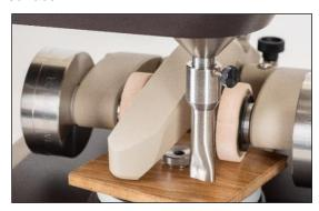
Using the Abraser touchscreen, enter the appropriate test parameter then press the "OK" button.
