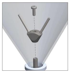
Lift the Taber vacuum pick-up nozzle into its upright rest position. Insert the offset, front orifice vacuum nozzle into the vacuum port opening.
