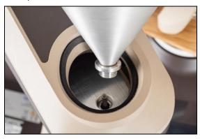
Insert the M3 Torx screw into the agitator hub; and then place the grit agitator on the agitator shaft inside the hopper. Secure by tightening the M3 Torx screw with the T-10 Torx Screwdriver.
