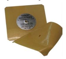
Mount the S-38 Standardization Plate to the Abraser specimen holder and lower the abraser arms.
