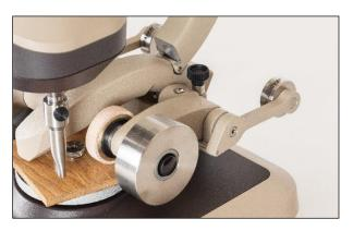
NOTE: The marking of the auxiliary weights indicates the total of both the weight and the abrading arm.
