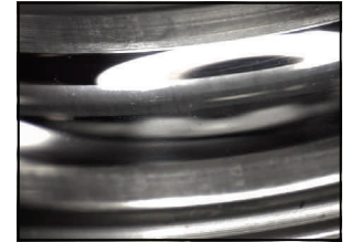
Solid band of fluting on the outer ring raceway
